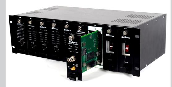
**Sunhillo's Longport** platform is a robust, versatile and modular system designed for Surveillance Sensor Data Distribution and message conversions and now with the addition of the **ADS-B Receiver** module it accepts and decodes 1090MHz and 978MHz ADS-B and TIS-B.
